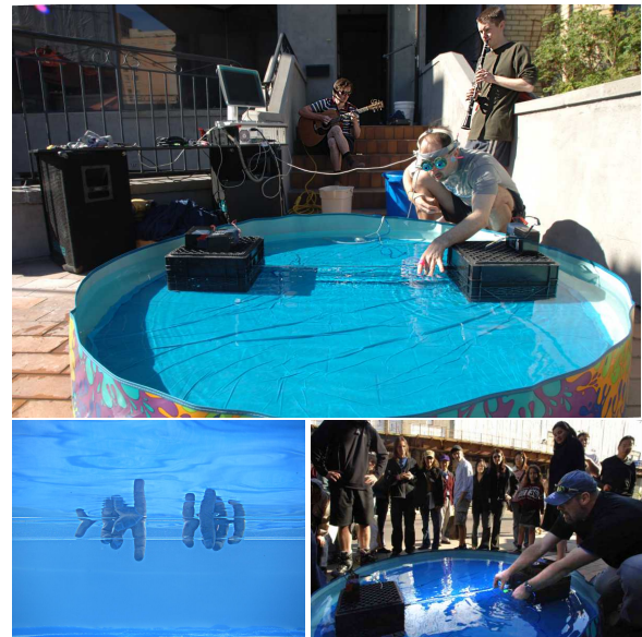
Figure 8. An underwater friction-idiophone based on total-internal reflection: Underwater (plus optional overhead) cameras “look” at a glass cylinder. Placing the camera further underwater than the cylinder, and having it look up at an angle, makes it possible to see the fingers as they disturb the evanescent wave of total internal reflection. This gives rise to a hyper-sensitivity in the image plane, making visible subtle sound-induced ripples in the water that occur from sound vibrations in the glass cylinder. With carefully constructed computer vision, the camera can thus function as an optical pickup of acoustic phenomena, much like an electric guitar having an optical pickup. Together with an array of geophones, hydrophones, and microphones, this provides a multiply acoustic instrument having a richly acoustic physicality.
