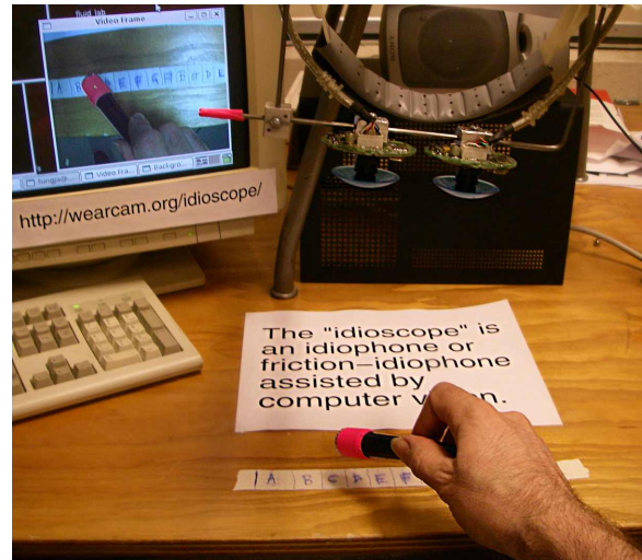
Figure 4. Making a bell-like sound from hitting a desk: A computer music system that is not an electronic instrument. Sound originates acoustically, and the role of the computer is merely for post-processing (much like a Wah Wah pedal on a guitar). The center frequency of the filter's passband varies with position, as detected by the overhead camera rig. Note the wearable stereo camera rig hanging from a fixed location. The cameras can be mounted to a tripod, or worn by the player.
