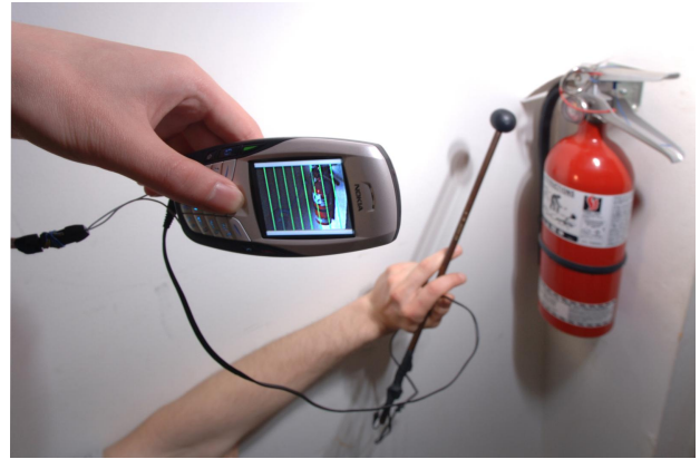
Figure 6. A 12-bar idioscope running on a camera phone: One or two drumsticks or mallets with contact microphones plug into the headset input of a standard cameraphone. While listening to earphones, the player strikes an object in view of the camera. There are 12 vertical zones, each defining a separate note on the musical scale. The player can walk down the street and strike street signs, lamp posts, and the like, as part of a live performance webcast in real time. Here the player is locating a fire extinguisher through one of the 12 zones defined in the camera phone view and hitting the extinguisher with the mallet. Whatever pitch is produced by the sound of hitting the extinguisher is filtered and frequency-shifted to the desired note, so that all 12 notes can be produced by hitting this one fire extinguisher or other similar everyday objects.
