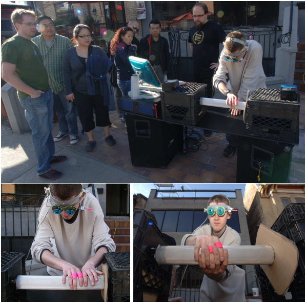
Figure 7. Polyphonic friction-idiophone having continuously variable pitch: A spinning aluminum cylinder with a specially textured surface produces sound picked up by a wireless contact microphone inside the cylinder. The sound is fed to one or more (depending on the number of fingers touching the cylinder) bandpass filters controlled by computer vision. The instrument can be used above or below the surface of the water.
